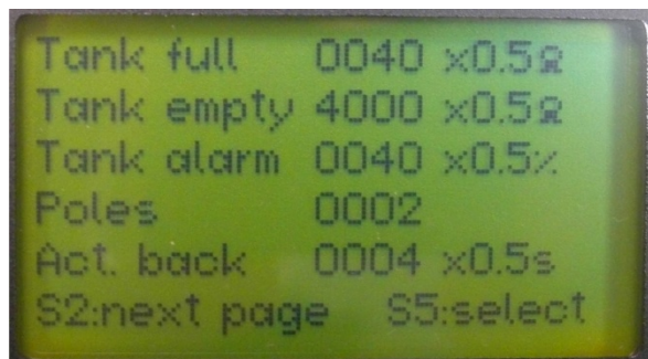
Figure 23: Resistance for tank sensor and alarm level
